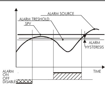
This alarm is desabled at the starting of PL300 and it is automatically activated when the alarm source exceeds the alarm treshold of a value which is equal to the hysteresis. Then the alarm works like the above described "deviation low alarm".
