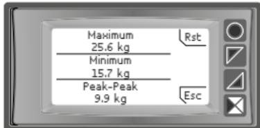
The STR55X is provided with a page for the visualization of peak values: max. peak, min. peak and peak-to-peak of analogue input. Keeping pressed "Rst" it is possible to reset the visualized values.
