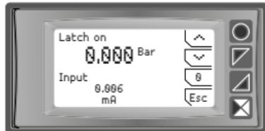
To use the LATCH ON function: enter configuration, select **Setting** on par. 8 **Latch on** and press "Sel" (STR55X shows the page in the picture).
