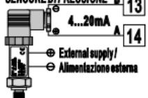
For linear signals 0/4..20 mA with **external power of sensor**.
