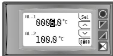
Press "Setpoint" to enter the thresholds modification.
