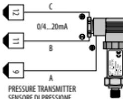
For signals 0/4..20mA with **three-wire sensor**
