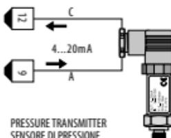
For signals 0/4..20mA with **two-wire sensor**
