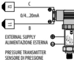
For signals 0/4..20mA with **external power of sensor**
