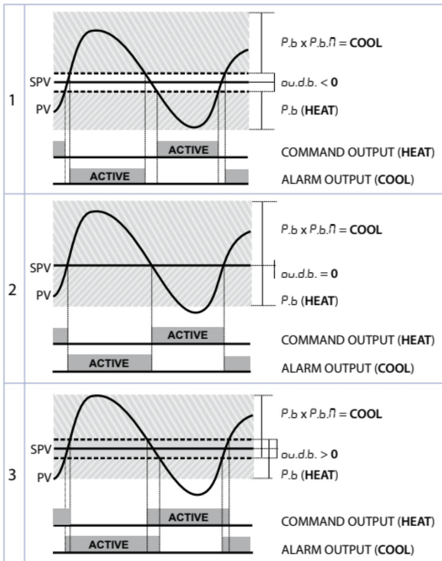
Parameter  $t.c.2$  has the same meaning of the cycle time  $t.c.$  for heating. Parameter  $co.F$  (cooling fluid) pre-selects the proportional band multiplier  $P.b.\Pi$  and the cooling PID cycle time  $t.c.2$  basing on the type of cooling fluid:
