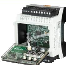
The internal display, in combination with the pushbuttons **▲**, **▼** and **SET** is used to configure the module. In the power on phase the display shows the firmware version while in normal operation, in the absence of anomalies, the display remains off. In case of anomalies it shows the number of the active error. In the configuration phase it shows the parameter being entered.
