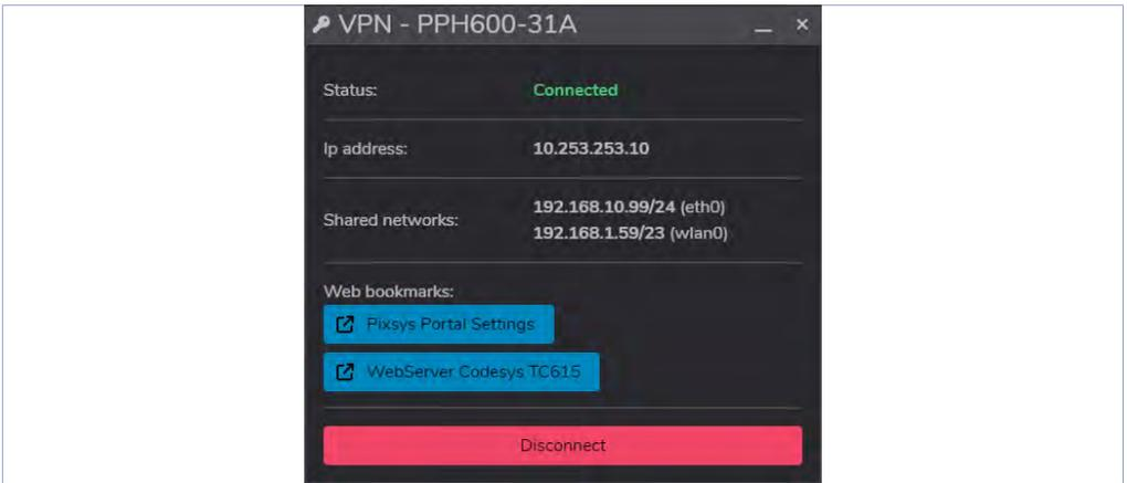
Clicking on “Disconnect” terminates the WebRTC connection from the gateway. Instead, clicking on the “VPN” button and then on “Connect” displays the window showing the buttons giving access to the various configured WebServers (see section 6 “Web Bookmarks” in the first paragraph for more information). You will also see the IP address assigned to that device and the information of the accessible networks (see section 3 “Network” of the first paragraph for more information).
