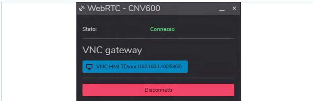
Pressing on the "Direct Control" button and then on Connect displays the window showing the buttons giving access to the various configured VNC servers (see section "VNC gateway" for more information).
