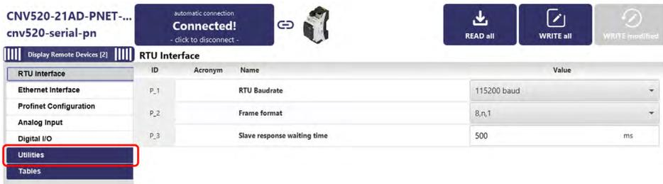
The screenshot shows the RTU configuration interface for a CNV520-21AD-PNET device. The device is connected via an automatic connection. The interface includes buttons for 'READ all', 'WRITE all', and 'WRITE Inmodified'. Below these is a table of RTU Interface parameters:
