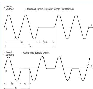
For a percentage less than 66%, SSR output firing takes place as in the "Burst fire" mode. (parag. 7.12.b)
