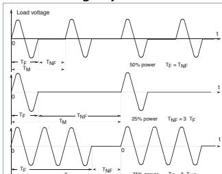
**At 50% power, the modulation time is 40ms:**
