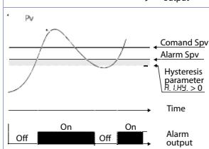
Upper deviation alarm value of alarm setpoint less than "0" and hysteresis value greater than "0" (Par.58 R.I.HY > 0).
