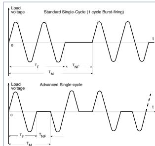
For a percentage less than 66%, SSR output firing takes place as in the "Burst fire" mode. (parag. 9.b)
