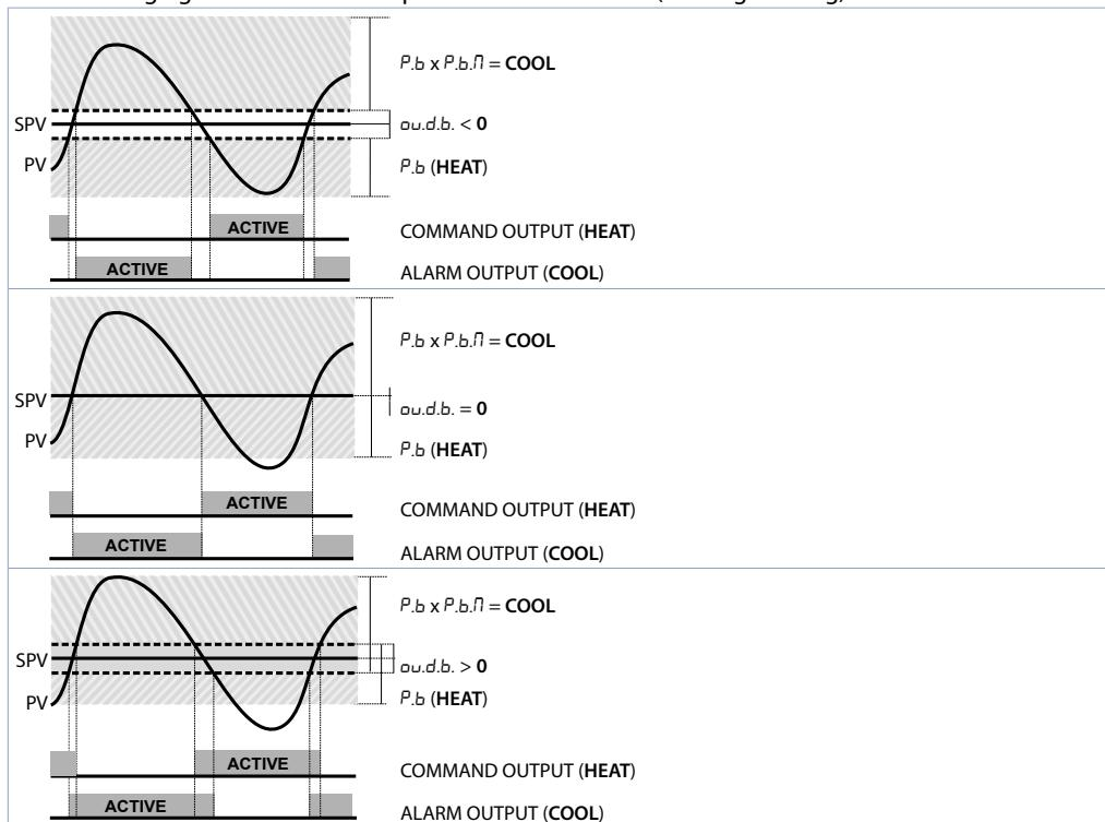
The parameter *coo.F.* has the same meaning as the heating time cycle *t.c.*
