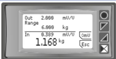
Press “mV” to go back to setting of mV/V ratio.
