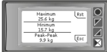
The STR561 is provided with a page for the visualization of peak values: max. peak, min. peak and peak-to-peak of analogue input. Keeping pressed "Rst" it is possible to reset the visualized values.
