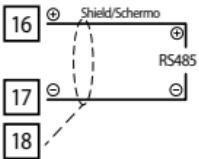
RS485 Modbus RTU communication
