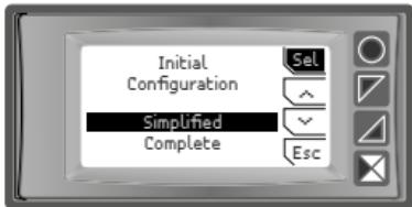
Once selected the language, it is possible to choose between two configuration modes: simplified or complete. The first mode allows to enter directly the parameter of pre-selected Easy-Up configurations, while selecting the second option it is possible to enter the complete configuration menu. "Esc" cancels configuration procedure.
